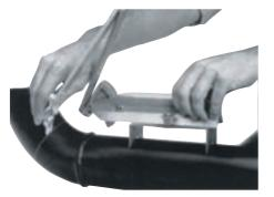
Designed for use with the Standard and Jumbo Contour Markers, the adaptor simplifies handling and increases layout flexibility.Permits use of all four sides of the Contour Marker and allows marking on small diameter pipe, over nipples, old weld or on wrapped pipe. Also provides layouts with compound angles Using a single setting, or any degree of take-off on elbows and turns up to 90°.
