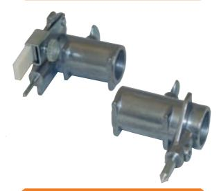
Using standard half inch pipe as a trammel bar, heads feature radius set points cast in alignment with marking pointers for easy setting. Equipped with 1/4" screws and squared on the back side of perpendicular alignment. The stationary head holds a 1/4" case hardened center point. Moveable head has a 1/8" steel scribe hardened. Marks from 1-1/2" circle to any diameter needed, depending on length of pipe used as a trammel bar. Allen wrench, soapstone, scribe and pointer also included.
