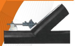
$90^{\circ}$  protractor has a matching locking lever to set and hold the tool at the desired angle. Equipped with a 5.8" by 10" tapered arm to complete finding of angles or desired bends, or to determine any portions of elbows. Tool is mounted in a 3/4" wide frame with a 3/8" by 6" cast-in rod and comes with a 25-pound pull magnetic base for holding the protractor frame in position. Can be used manually or with a magnetic base.
