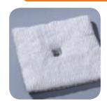
These flexible pads are made from special non-asbestos, resilient, high temperature materials. Non-combustible and chemically inert, they provide temporary insulation of welds during stress relieving of large diameter piping, ducts, vessels, or tanks. Available in 12", 24" or 48" widths and 1", 1.5", and 2" thicknesses.
