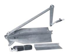
Developed for use in the layout of large diameter pipe, from 8" to 48" and structural seal joints, of the same size pipe. Comes complete with a durable web strap (included) to help hold the unit in place during layout. Built-in adjustable dial set level (DSL) ensures accurate center-line location. A soapstone crayon is included.
