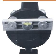
Designed primarily for pipe fitting applications, the Universal Level is a valuable tool for any craft required to use a level or a plumb bob:
